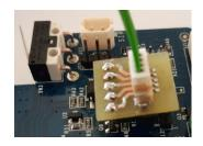
Connect the test capsule to the motherboard smoke canister connector.
